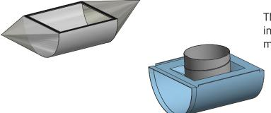
The T-SRD is fastened to the inside of the fabric duct by means of velcro
