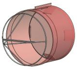
Insert the SafeStretch Ring into the SafeStretch Bottom and fix it with the push buttons (or for sizes bigger than 24") the rubber ring.
