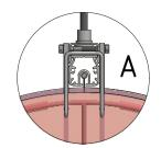
For ducts larger than 24" diameter a hook is supplied to stabilize the SafeStretch Ring/Bottom.
