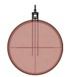
Use the SafeStretch Bracket to stretch the fabric duct by sliding the bracket towards the end of the duct till the duct is taut. Then tighten the grub screw.
