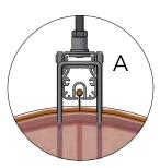
For ducts larger than 600 mm diameter a hook is supplied to stabilise the SafeStretch Ring/Bottom.
