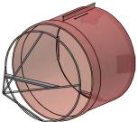
Insert the SafeStretch Ring into the SafeStretch Bottom and fix it with the push buttons (or for sizes bigger than 600 mm) the rubber ring.
