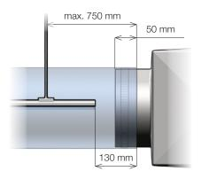
The SafeTrack is supplied in cut lengths to match the textile duct and is packed with the necessary components and marked individually with exact indication of placement.
