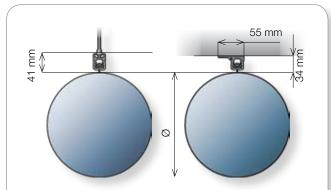
SafeTrack is clicked directly into the **SafeCeil** for convenience and is designed for mounting the textile duct close to the ceiling.
