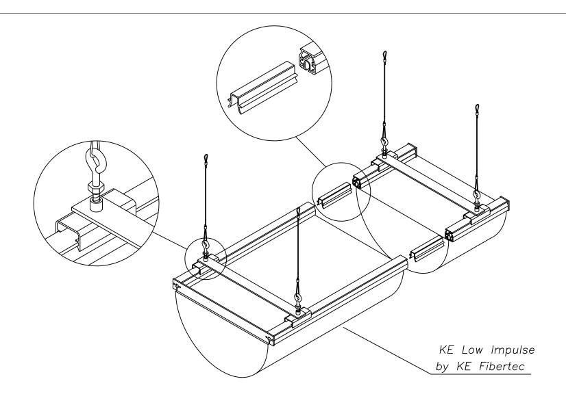
Snap on suspension section with cable insert
