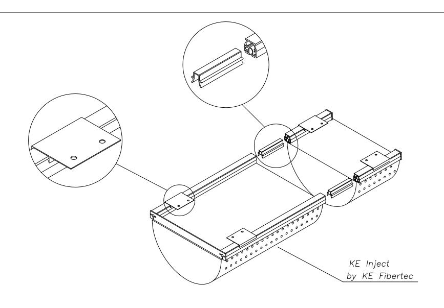
Safe Track with Flush Mount for KE Fibertec Half-Round Fabric Ducts
