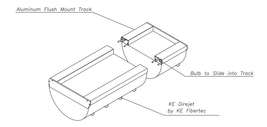
D-Lite Alu Suspension for KE Fibertec Half-Round Fabric Ducts
