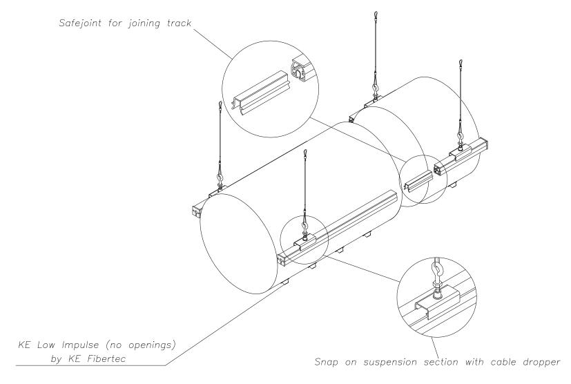
Dual Track Suspension Detail for Fabric Ducts (3 and 9 o' clock Attachment)
