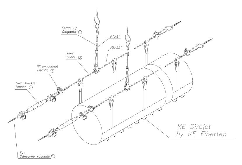
Double Cable Suspension Detail for Fabric Ducts (12 o' clock Attachment)
