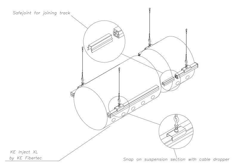
Dual Track Suspension Detail for Fabric Ducts (3 and 9 o' clock Attachment)
