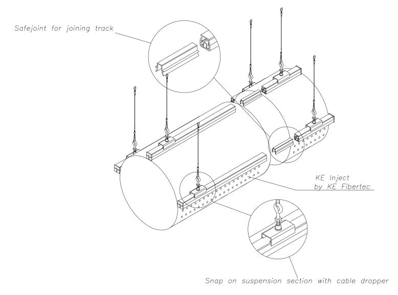
Triple Track Suspension Detail for KE Fibertec Fabric Ducts (3, 9 & 12 O'clock Attachment)
