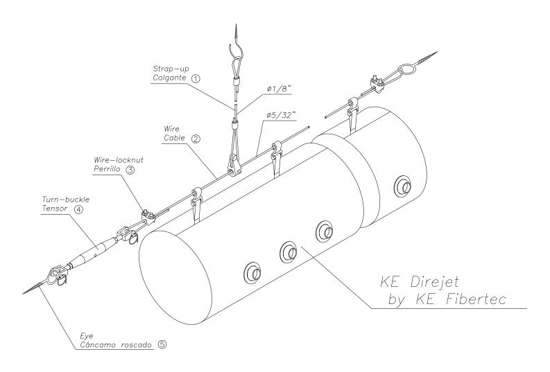
Single Cable Suspension Detail for Fabric Ducts (12 o' clock Attachment)
