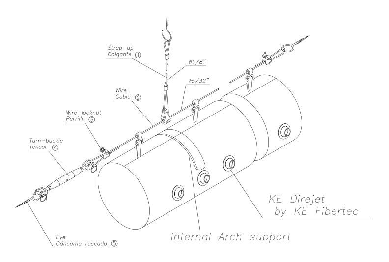
Wire Arch Suspension Detail for Fabric Ducts (12 o' clock Attachment)
