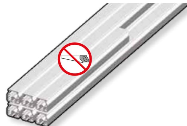
Alu-rails labelled with a saw symbol do not require further trimming.
