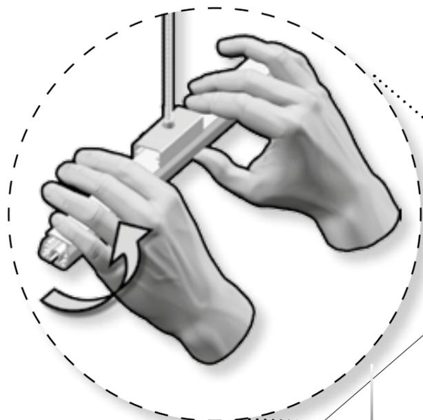
**1** Supports and spacing profiles are mounted on the ceiling; positioned in accordance to the location of inlet socket, duct start or duct bottom.
