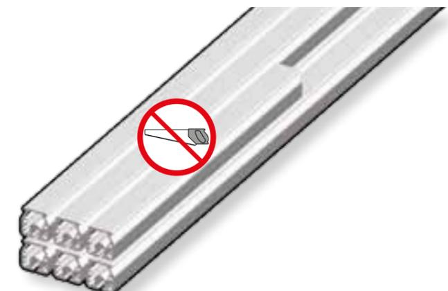
Alu-rails labelled with a saw symbol do not require further trimming.
