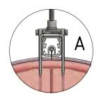
For ducts larger than 600 mm diameter a hook is supplied to stabilise the SafeStretch Ring/Bottom.
