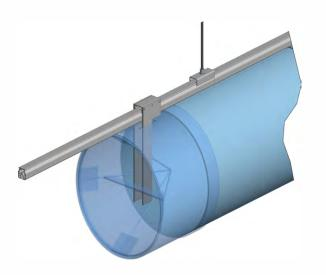
The SafeStretch<sup>®</sup> system will keep the textile duct round and taut at all times with or without air pressure.
