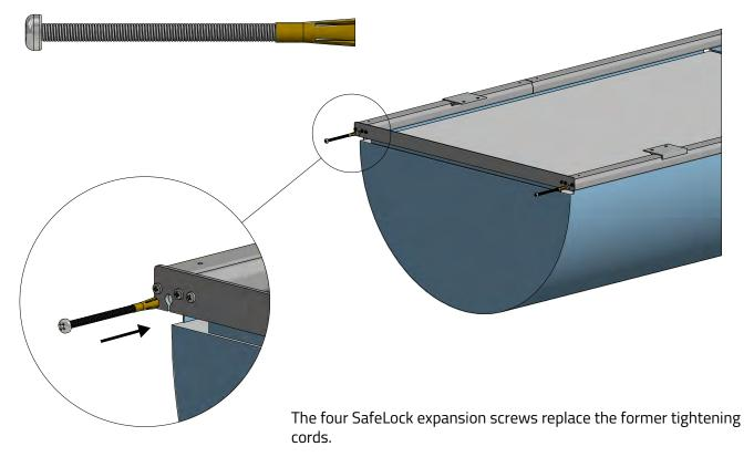
The SafeLock is inserted into the "keyhole" at the end of the Safetrack. Apply drill driver with bit PC2.
