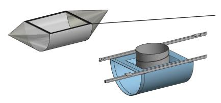
The T-SRD is fastened to the inside of the textile duct by means of velcro
